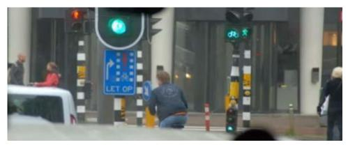
Figure 2.4.2 Example from the Netherlands of traffic signals + give way signage controlling turning traffic and cyclists (Source: Dutch Design Guide Ontwerpwijzer Fietsverkeer)
